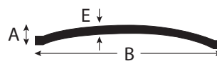
MEDIA CAÑA DE ACERO STAINLESS STEEL JOINT COVER DEMI BOMBÉ EN ACIER INOXYDABLE
